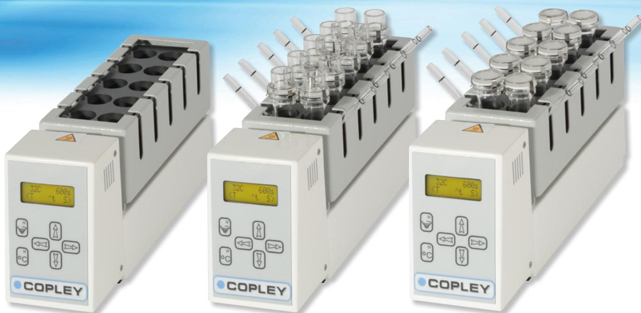
Vertical Diffusion Cell Test System Model HDT 1000 (without cells, with "open" cell tops and with "occluded" cell tops)
