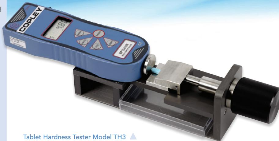
Tablet Hardness Tester Model TH3 ▲
