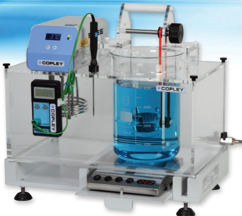
The Suppository Tester SDT 1000 is a single stage unit which has been designed in accordance with the specifications as laid down in the **Ph.Eur. Test 2.9.2 for the disintegration of suppositories, pessaries and vaginal tablets** and with suitable attachments **2.9.22.-2 Apparatus 2 for measuring the softening time of lipophilic suppositories.**
