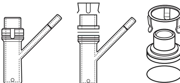
Cell Type C with "Open" Cell Top together with exploded Cell and Sample Holder
