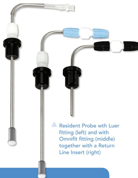
▲ Resident Probe with Luer fitting (left) and with Omnifit fitting (middle) together with a Return Line Insert (right)
