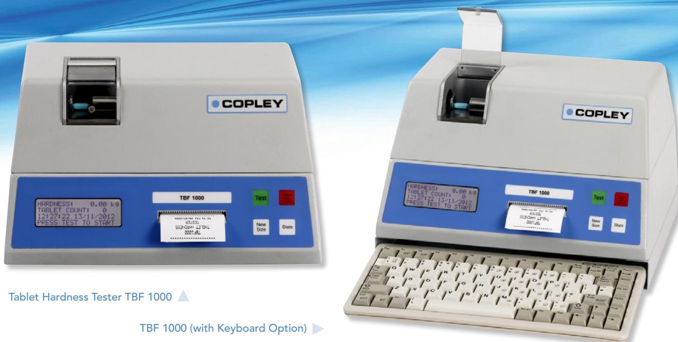
Tablet Hardness Tester TBF 1000 ▲
