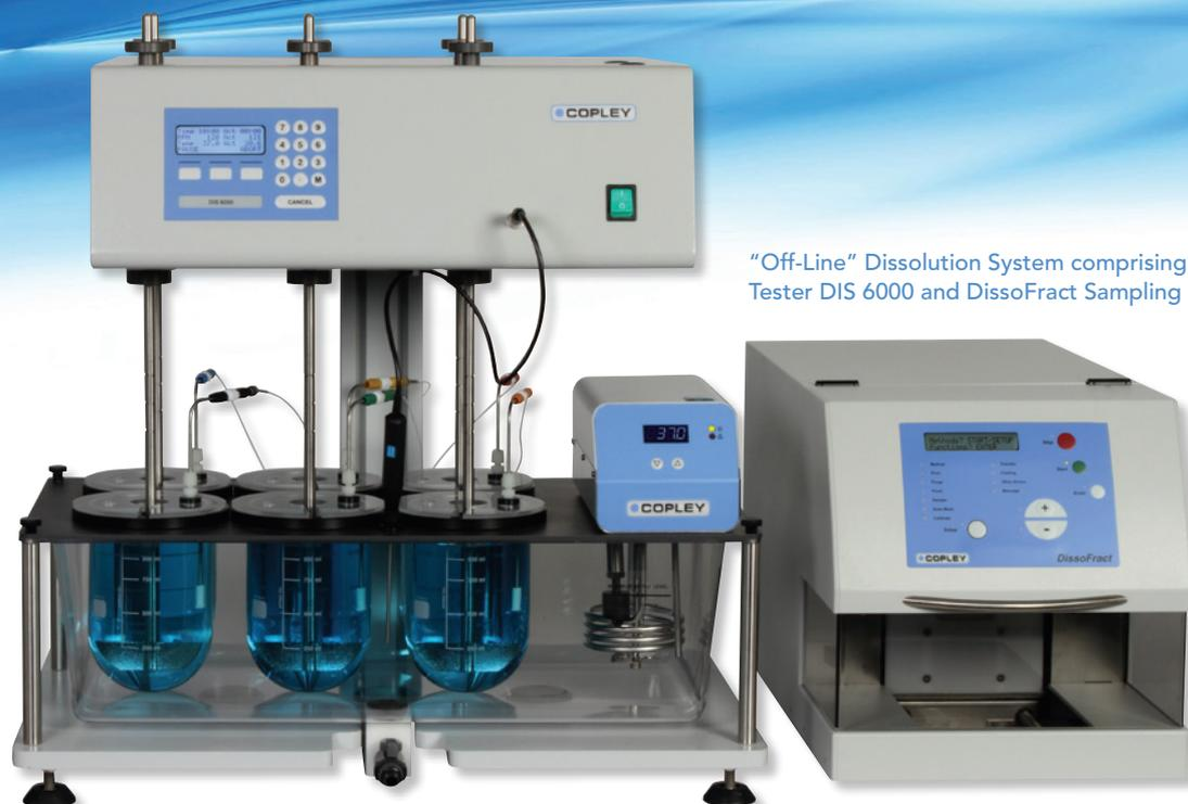
"Off-Line" Dissolution System comprising Dissolution Tester DIS 6000 and DissoFract Sampling System
