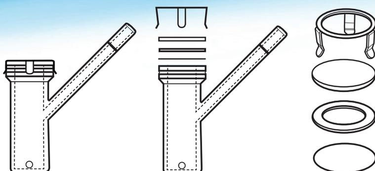
Cell Type "C" with "Closed" Cell Top together with exploded Cell and Sample Holder
