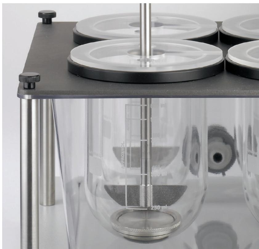
Membrane Holder in Dissolution Vessel ▶
