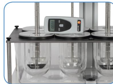
Shaft Rotational Speed (Tachometer)
