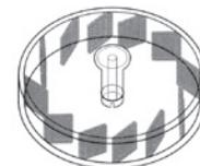
Schematic of Abrasion Drum
