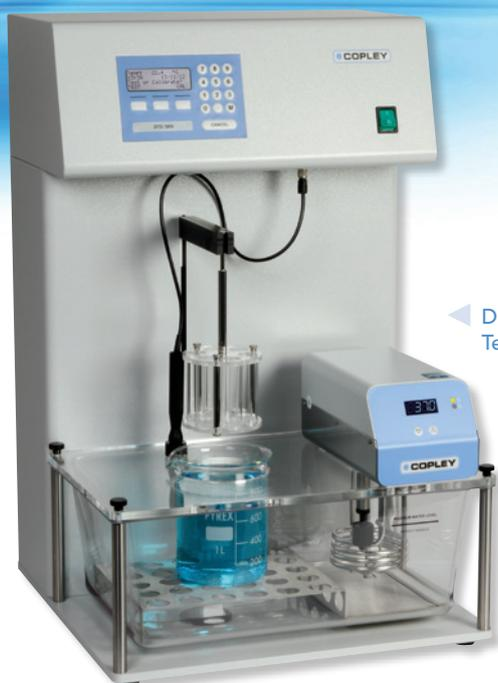
◀ Disintegration Tester DTG 1000
